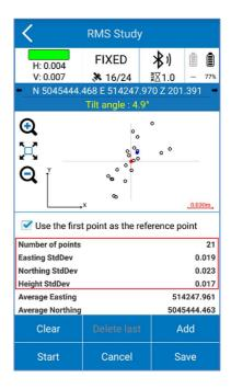
The user has the control of the number of sample positions used in the RMS calculation. When the user decides to complete the check, he can press **Stop** to stop the automatic position acquisition.
