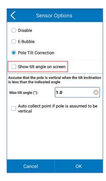
The user can also define the verticality tolerance of the instrument.
