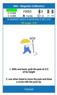
The second screen lets the sensor adjust the calibration parameters based on the local GNSS position and accuracy.
